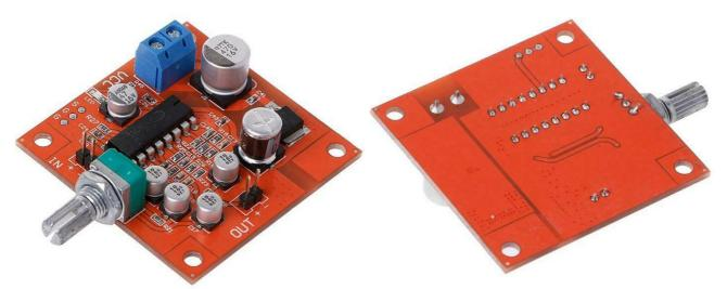
This module can be bought from Ebay and AliExpress for just a few dollars. The circuit on this board is similar but *not identical* to the echo circuit from the PT2399 datasheet.
