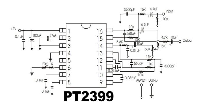
The module needs some minor modifications. The onboard feedback pot was removed, as was the power terminal block, plus the input and output header pin terminals. The existing resistor between pin 6 and earth (labled "R27") was removed. The amount of resistance between pin 6 and earth controls the internal oscillator and therefore the delay time. The datasheet has a table of values and delay times. Note the increase in distortion (THD) as the time (td) increases.
