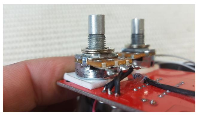
The delay time pot was installed in a similar way, with the anticlockwise lug wired straight to the vacant earth pad from the removed output signal connector. The 2.2k resistor was wired directly from the pin 6 solder pad (labelled "s") to the middle and clockwise lugs of the delay time pot. The resistor was held in place with a drop of hot glue, and the long leg was covered in a length of heatshrink to prevent shorting to the IC legs. The pots can now be used to mount the module.
