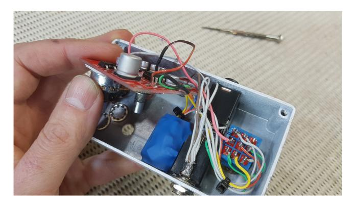
Here's the wiring diagram. The 100k resistor (R5) was mounted on the stomp switch.
