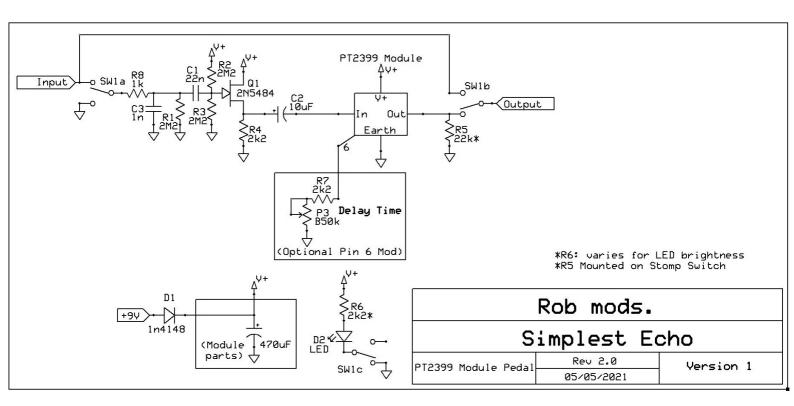
The slight (~0.5dB) loss through the buffer is made up by the module with its ~1dB of gain, so I chose to omit a volume control, as the pedal would be very close to unity gain.
