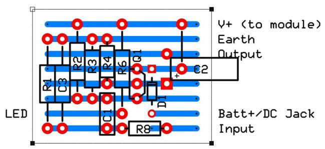
It was encased in heatshrink, and installed with double-sided tape to the underside of the top of the enclosure between the pots and the jacks. The module is placed over it. For this reason, the output coupling cap (C2) was placed on its side.
