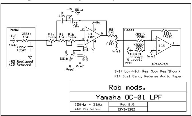
C5 was removed, and R5 was replaced with a 15k resistor which becomes part of the new filter. The original "Direct Level" pot was removed, which leaves R32 dangling. This essentially converts IC5's first op amp from a virtual earth mixer, to an inverting buffer with a 220k input impedance. I also repaced the "Effect Level" pot with an A10k pot as a master volume. The 8.2k resistor (R2) attenuates the signal by 5dB.
