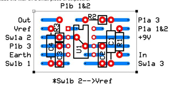
It is only 15mm wide to fit in the pedal. I also used small MKT caps to keep the height below 10mm, since the top half of the enclosure is only 13mm deep.
