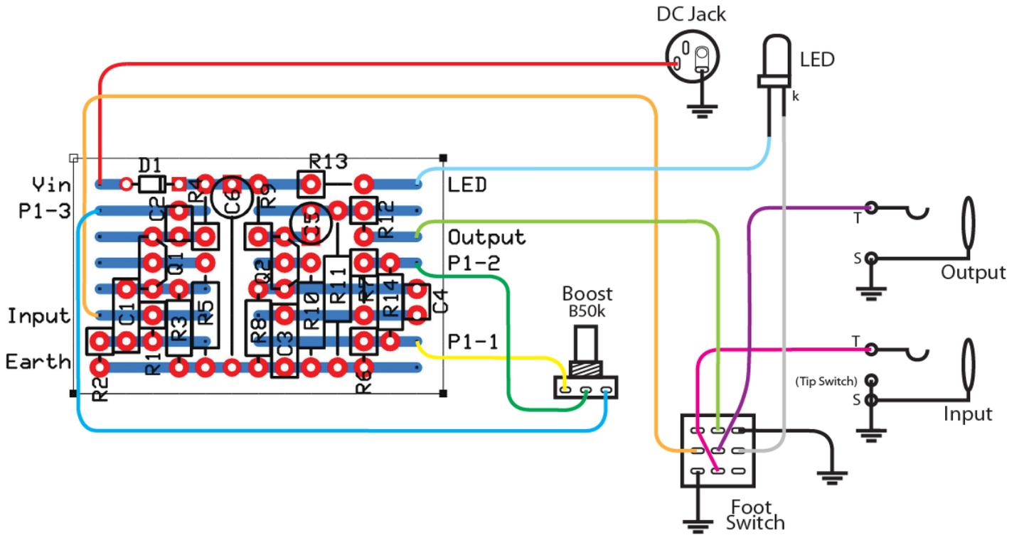
With the low profile jacks I used (Altronics #P0097), and the 9mm pot, it was relatively easy to fit the circuit and parts into the small enclosure (Hammond 1590A style).
