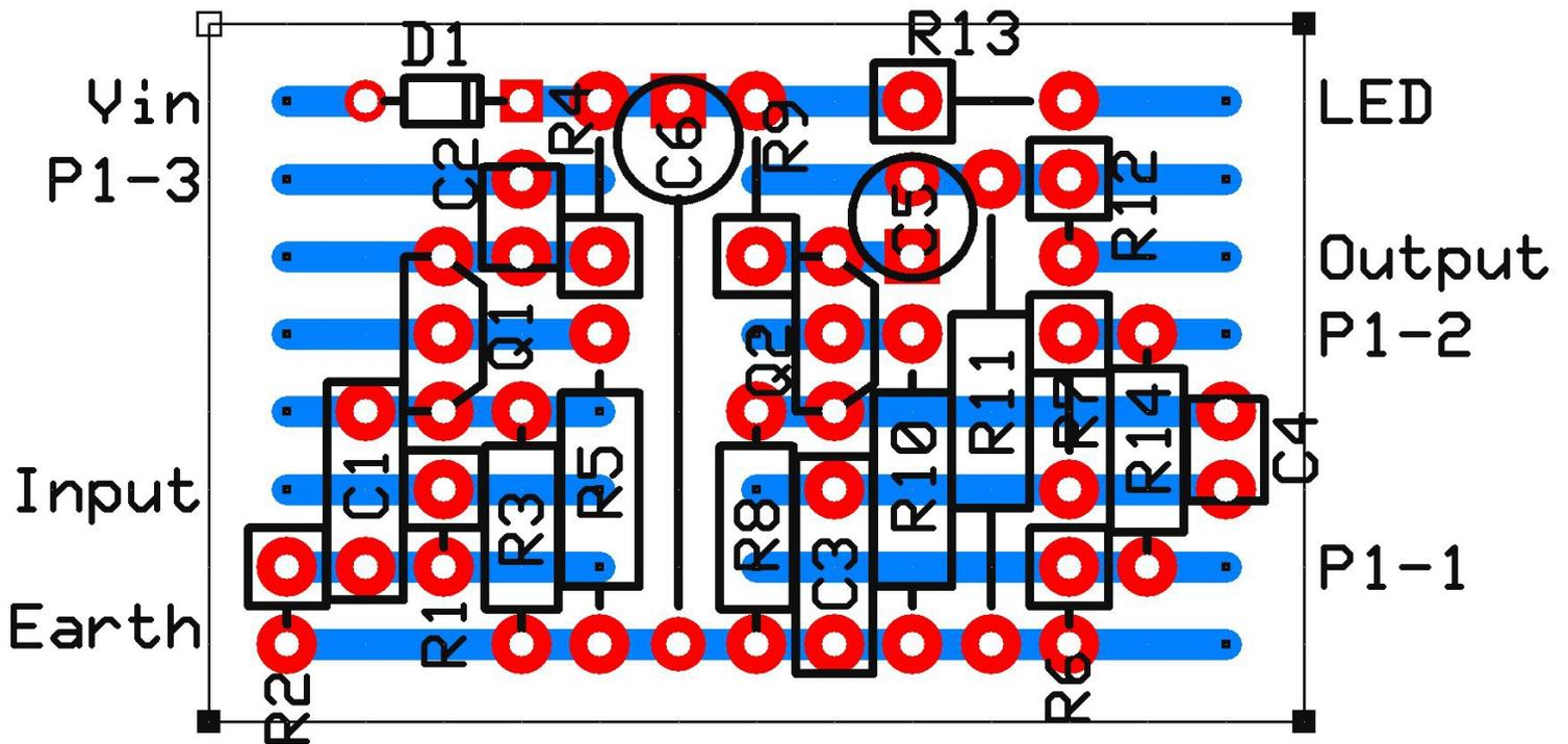
It is only 34mm x 21mm. The parts are fairly cramped, and several resistors have to be installed standing up. C2 should be a monolithic type. C4 is preferred as a monolithic, but other types could be used with their legs bent underneath slightly.
