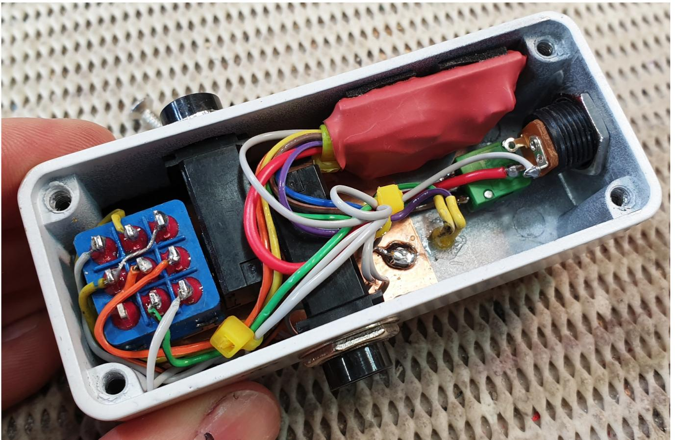
For my prototype, I used a pre-painted white enclosure. The white finish was poor and I needed to rub it back with 1200g to remove excessive orange peel and quite a few specks of grit in the paint. For the graphics I used water transfer decal sheet.
